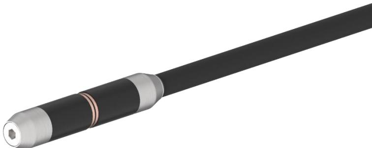
*Ex: TECT-200-MF2-A2-095-25M04 → ECT bobbin probe rigid with cable, OD 20 mm, Mid frequency MF2 (250 kHz), Tube type A (Nylon), Without retrieve cable, Pushing Tube OD 9.5 mm (3/8"), Cable length 25 m (80'), 4-pin connector.*
