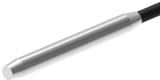
E.G: **TNFT-200-LF2-20M19** → NFT bobbin probe, OD 20 mm, Mid Frequency LF2 (75 Hz), Cable length 20 m (65'), Connector 19 pins
