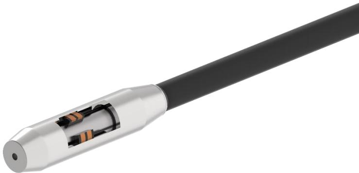
**E.G. TSAT-112-MF1-A2-079-20M04** → ECT saturation bobbin probe rigid with cable, OD 11.2 mm, Mid frequency MF1 (100 kHz), Tube type A (Nylon), Without retrieve cable, Pushing Tube OD 7.9 mm (5/16"), Cable length 20 m (65'), 4 pins Amphenol connector
