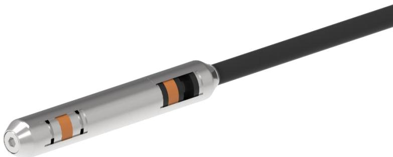
E.G: **TRNF-200-LF2-20M19** → RFT & NFT probe, OD 20 mm, Mid Frequency LF2 (75 Hz), Cable length 20 m (65'), Connector 19 pins
