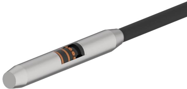
E.G: **TNFA-200-LF2-20M41** → NFA bobbin probe, OD 20 mm, Mid Frequency LF2 (50 Hz), Cable length 20 m (65'), Connector 41 pins
