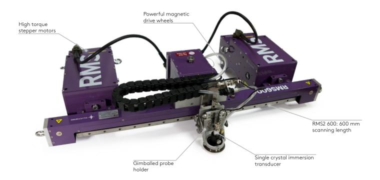
RMS2 can give 100% coverage in a band up to 1000 mm wide, significantly increasing Probability of Detection (POD) of defects and corrosion, enabling engineers to determine the optimum repair strategy and improve remaining life assessment (RLA) & risk based inspection (RBI) maintenance programs.
