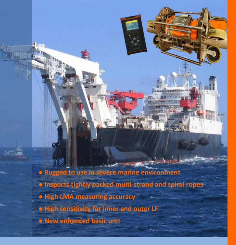
Wire ropes for offshore heavy lifting usually have large diameter, and their length may exceed 2000 m. These high-value ropes may have multi-strand construction, and require proper non-destructive inspection in order to extend their safe operation as long as possible. Based on long time experience with magnetic rope testing, Intron Plus has recently developed equipment for inspection of wire ropes with diameter up to 175 mm for a wide variety of applications.
