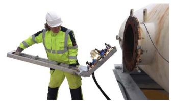
Deployment Crane for top- and side deployment
