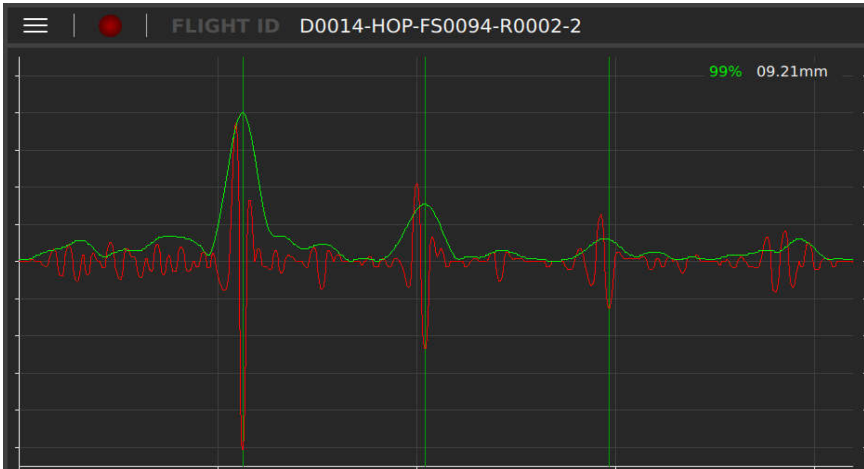
Bottom drone UT reading (9.21mm echo-to-echo)
