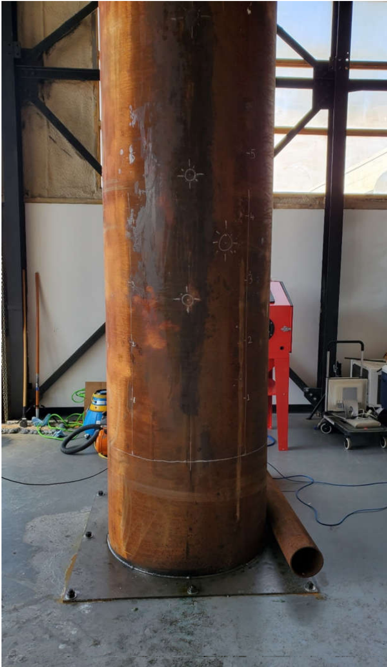
Layout of thickness reading locations (top, middle, bottom). Note middle location has visible signs of external wall loss.
