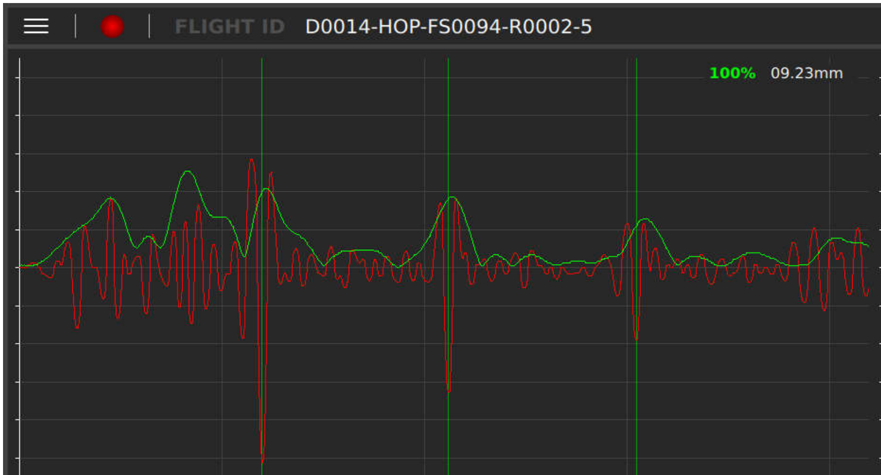
Top drone UT reading (9.23mm echo-to-echo)
