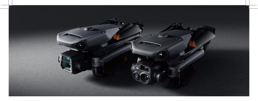
The Mavic 3 Enterprise redefines industry standards for small commercial drones. With a mechanical shutter, a 56× zoom camera, and an RTK module for centimeter-level precision, the Mavic 3E brings mission efficiency to new heights. A thermal version is available for firefighting, search and rescue, inspection, and night operations.
