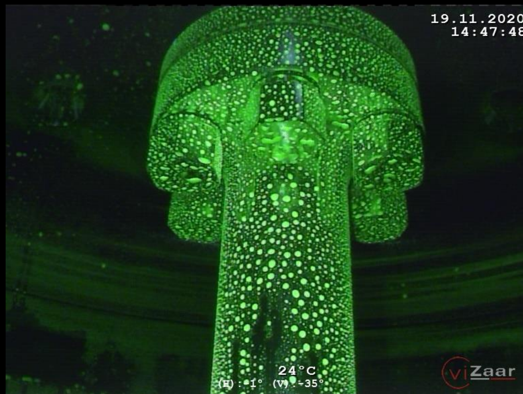
Fluorescent riboflavin inspection with UV radiation
