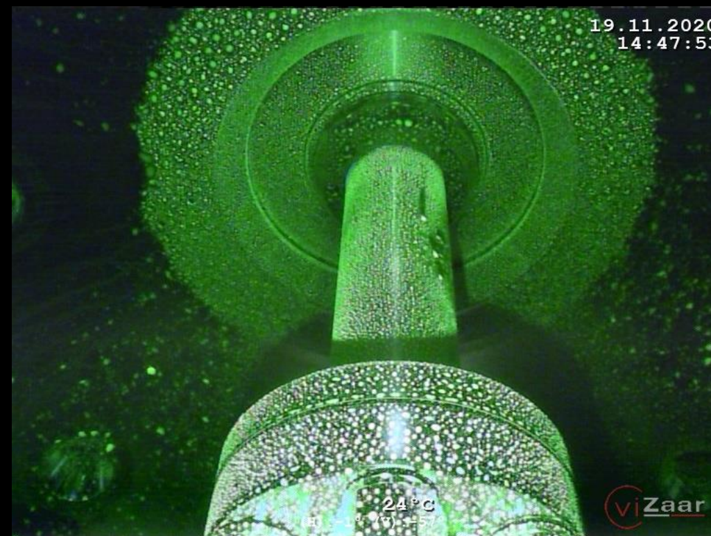
Fluorescent riboflavin inspection with UV radiation
