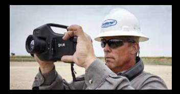
Optical gas imaging allows you to work from a safe area to scan for signs of hazardous gas plumes. Then, move in closer to begin your complete inspection. Survey hard-to-reach connections and fittings without the risk of placing yourself in harm's way. Once you find the exact location of a leak, repair work can proceed quickly.
