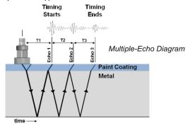
**Echo-Echo (Twin Crystal Probes)** measures through coatings of up to 1 mm (0.04 inch) thick, ideal for measuring painted metals with back wall corrosion.
