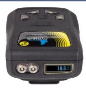
The Cygnus 2+ Hands Free thickness gauge uses multiple measuring techniques to accurately measure through coatings, as well as heavily corroded metals. The gauge has an end-mounted display and wrist strap, for hands free convenience.
