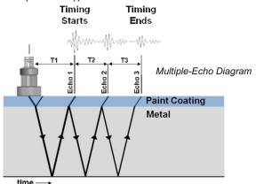
**Echo-Echo (Twin Crystal Probes)** measures through coatings of up to 1 mm (0.04 inch) thick, ideal for measuring painted metals with back wall corrosion.
