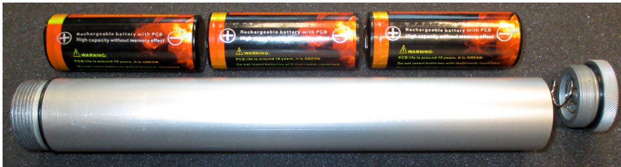
Camera battery tube with cover and battery pack in correct polarity (Minus towards the cover)
