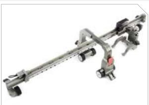
The Rotix – CEG027 is a manual chain corrosion scanner with a built in positional encoder and index encoder. It is designed to translate phased array probes and wedges around non-ferrous piping and vessels for the purpose of corrosion inspection. Urethane wheels built into the chain links provide smooth constant rolling when scanning. The Rotix chain can be adapted from 4 in. – 38 in. OD using multiple combinations of short and long links.
