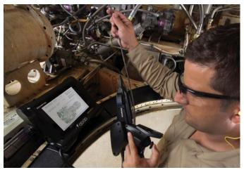
The IPLEX RX monitor displaying a manual PDF during inspection
