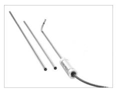
**Rigid Sleeve Sets** MAJ-1253 (for 6.0 mm insertion tube) MAJ-1737 (for 4.0 mm insertion tube) Sets are available for 6.0 mm and 4.0 mm scopes. Each set consists of three rigid sleeves of 250 mm, 340 mm and 450 mm lengths.
