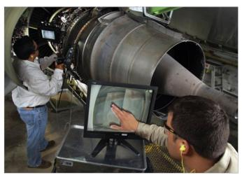
The same inspected image is shared between two operators with an external display connected to the IPLEX RX for remote observation
