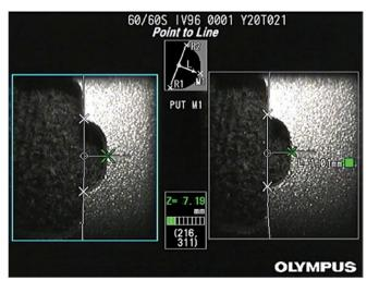
Stereo Measurement mode (Measuring the distance of a defect)
