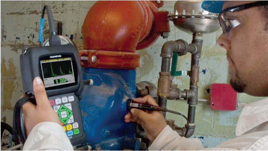
**Figure 1-1 Measuring thicknesses with the 38DL PLUS**
