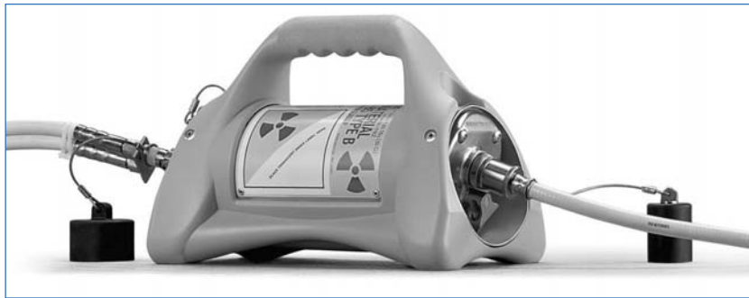
Fig. 15-5. S-channel container for Selenium75 with pigtail (at right) and operating hoses (at left)
