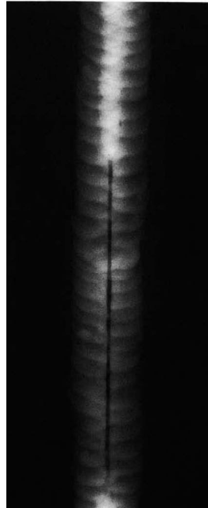
Incomplete - or Lack of Penetration (LoP) A darker density band, with very straight parallel edges, in the center of the width of the weld image.
