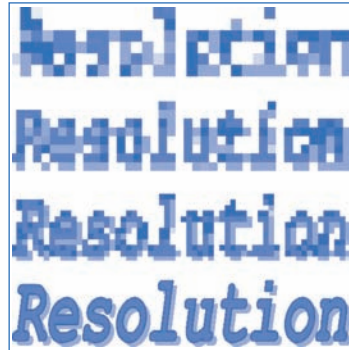
Fig. 26-16. Effect of number of pixels on lateral resolution
