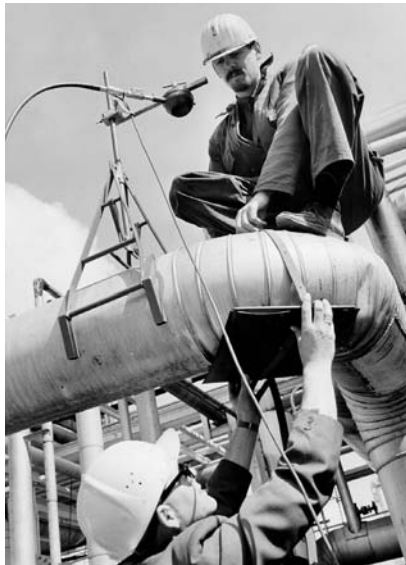
Fig. 8-18. Preparations for on-stream radiography
