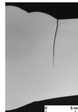
Macro of crack in a weld Fig. 18-17. Crack in austenitic weld
