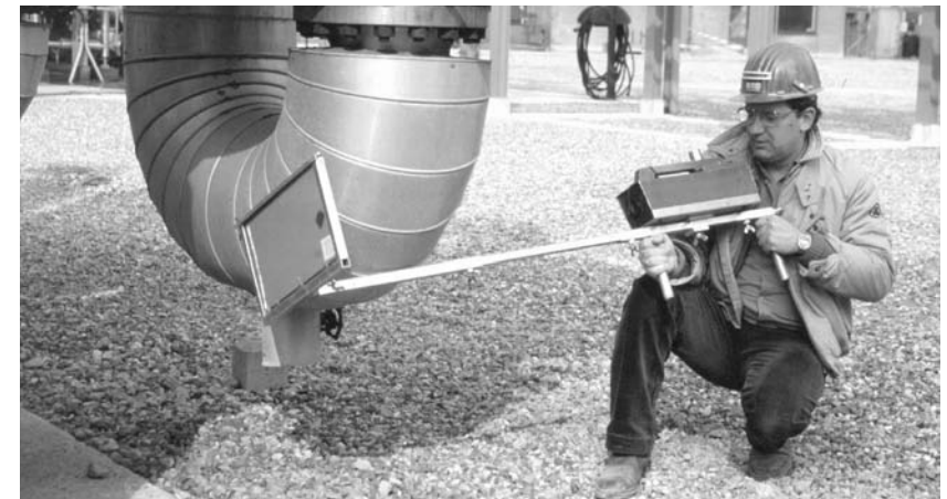
Fig. 10-18. Flash radiography of an insulated pipe section
