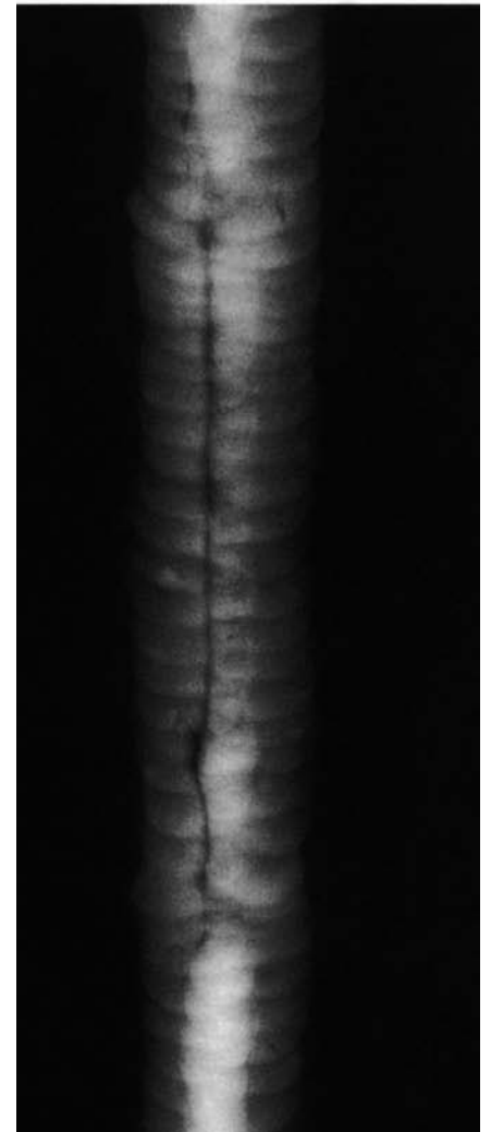
Internal (root) undercut. An irregular darker density near the centre of the width of the weld image and along the edge of the root pass image.
