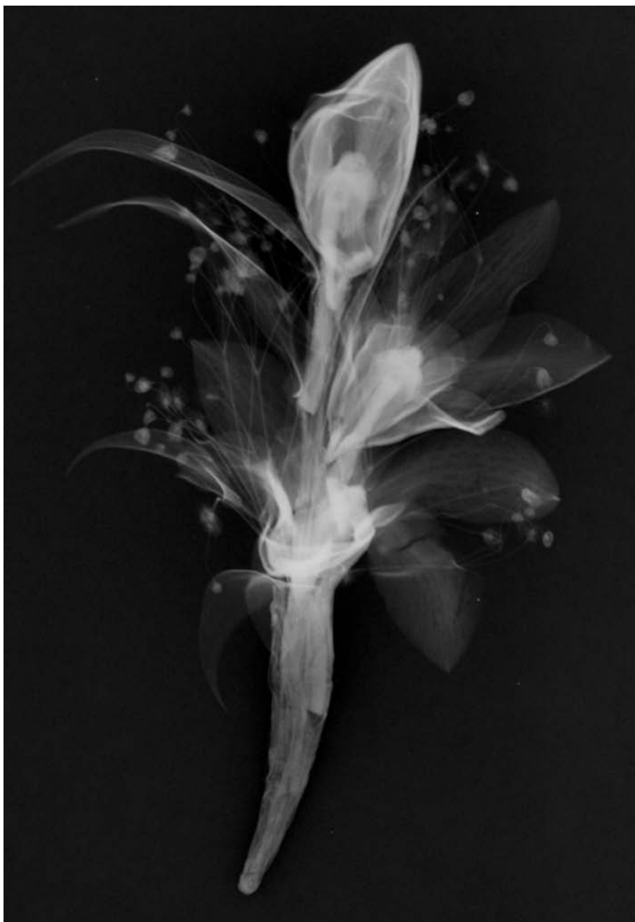
Neutron radiograph of an iris flower made on Agfa D3 s.c. (single coated) Organic substances are well suited to examination by this type of radiation.
