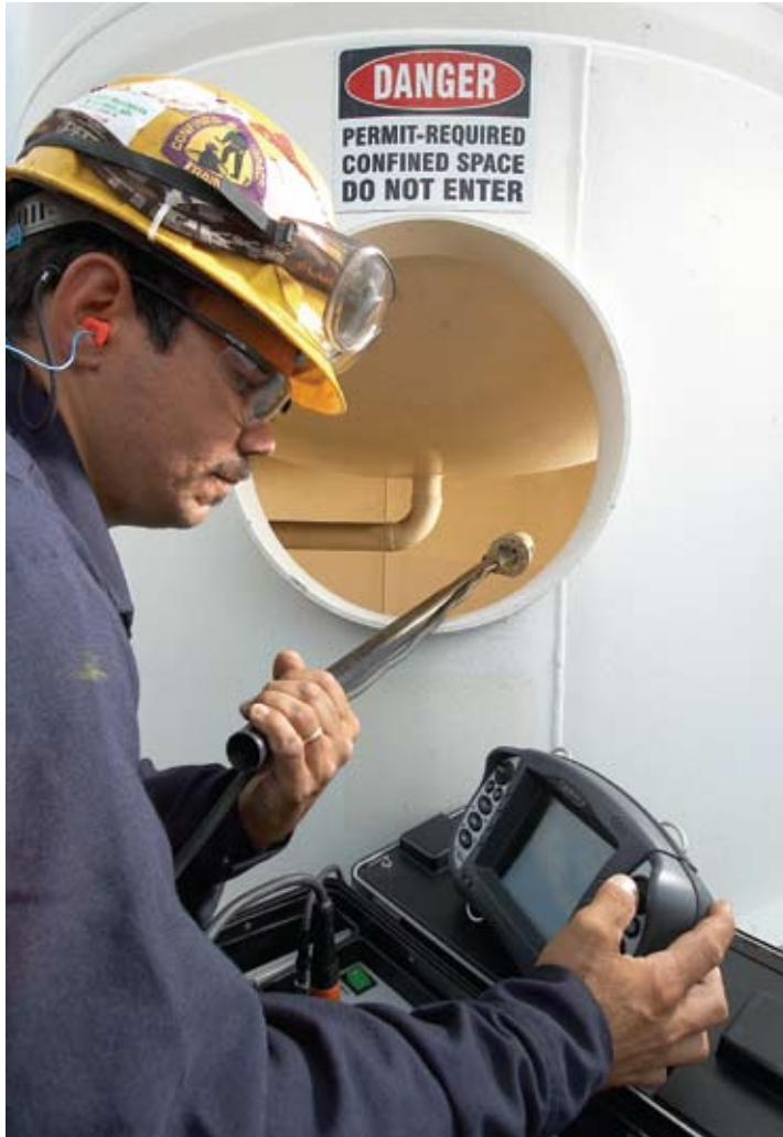
PTZ assists with confined space inspection
