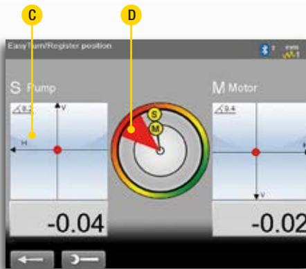
2. Take the measurement values in three positions with as little as 20° between. It is clearly visible on the display when the laser beam hits the detector.
