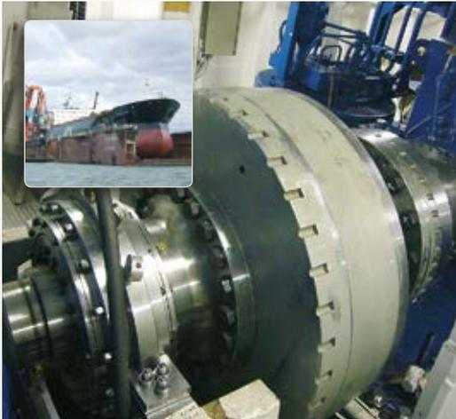
Engines, gearboxes and propeller shafts on ships are aligned using Easy-Laser® system. Thanks to versatile brackets you can install the equipment in the most appropriate place; shaft, coupling or flywheel.
