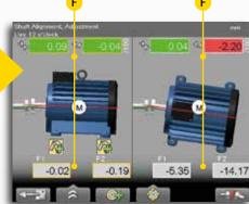
**3.** The live values reflect the adjustments made to the machine. For clarity, the adjustment is displayed both graphically and numerically. Horizontal and Vertical directions are shown at the same time.
